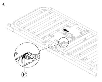
Cut all the zip ties **P** to release the wings, and fix the main module flat with the crossbars of the mattress support. Make sure new zip ties are placed in the same location when the main module is to be removed from the bed.
