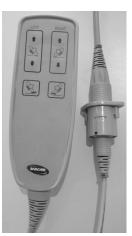
Connect the hand control to cable  ${\ensuremath{\mathbb R}}$  and connect the power cable 0 to the mains. The hand control cable is marked 3 on the cable clip corresponding to ③ on the control box cable.
