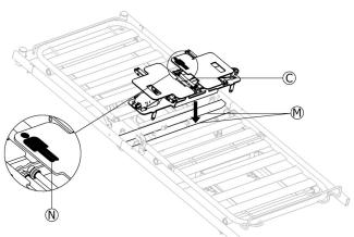
Place the main module C onto the crossbars M, following
