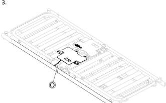
Ensure that the main module is placed in the middle of the mattress support frame and the distance <sup>(0)</sup>, to the side tubes is the same on both sides.
