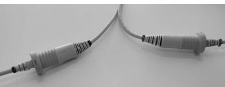
Connect the cables of the right and left motor to the two extension cables S and T from the control box. The right motor cable is marked 1 on the cable clip corresponding to 1 on the cable from the control box and the left motor cable is marked O on the cable
