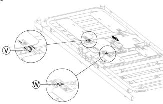
Ensure that the head arms are mounted on the telescopic bracket  $\ensuremath{\mathfrak{V}}$  in the first threaded hole and you are not able to see the remain-
