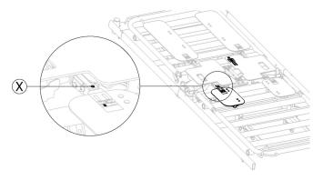
To adjust the position of the arms adjust the bolt <sup>®</sup> until the arms are in a horizontal position.
