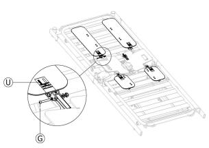
Connect the four arms with the main module, following the representation on the arms label shown in the zoomed image (0), the black shaded area on the sticker represents the location were the arm must be placed. Fix the four arms with the Allen bolts from set (6) and tighten the lock nuts facing inwards. Ensure the safety washers are placed on the lock nut side.
