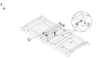
On each side of the bed, remove the nut  $\odot$  and bolt  $\circledast$  using two 13 mm keys to remove the slats assembly  $\odot$  from the bed, and keep it available for remounting, when the Soft Tilt is removed again from the bed.
