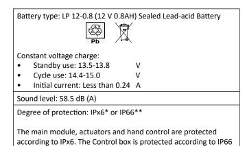
\* IPX6 classification means that the electrical system is protected against water projected from any direction (not high pressure).
