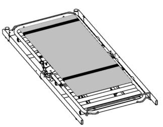
Mount the cover by sliding the pockets over the head end and foot end arms. The head end of the cover contains the label information and placement of the cover symbol:
