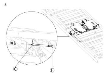
Fix the main module onto the crossbars of the mattress support frame, by placing the carrige-bolt (F), trough the designated bracket on the main module <sup>©</sup>, washer and nut, from underneath on both sides of the bed.
