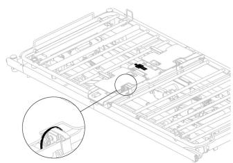
Cut all the zip ties to release the wings, before you start the motors. Make sure new zip ties are placed in the same location when the main module is to be removed from the bed.
