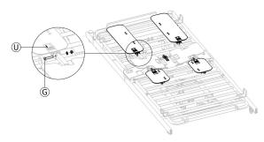
Connect the four arms with the main module, following the representation on the arms label shown in the zoomed image  $\bar{\mathbb{Q}}$ , the black shaded area on the sticker represents the location were the arm must be placed. Fix the four arms with the Allen bolts from set  $\bar{\mathbb{Q}}$  and tighten the lock nuts facing inwards. Ensure the safety washers are placed on the lock nut side.
