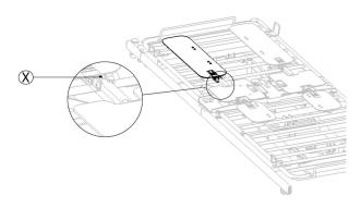
To adjust the position of the arms adjust the bolt  $\ensuremath{\mathfrak{V}}$  until the arms are in a horizontal position.
