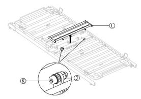
On each side of the bed, remove the nut 1 and bolt 8 using one 13 mm key and 6 mm Allen key to remove the slats assembly 1 from the bed, and keep all parts available for remounting, when the Soft Tilt is removed again from the bed.
