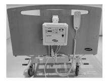
Collect the motor cables in a bundle and tighten it with a zip tie, move the bed up and down to make sure that the bundle is not clinging on any bed parts and moves freely.
