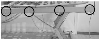
Run the motor cable underneath the bed frame toward the foot end, on both sides of the bed and fix each of the cables with zip ties onto the frame tube. Ensure that both motor cables are tighten with zip ties (marked by the circles in the picture), first zip tie near the motor and the last 3 on the frame tube toward the foot end. Make sure the end of the zip ties, are not facing outwards from the bed frame.
