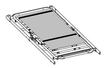
Mount the cover by sliding the pockets over the head end and foot end arms. The head end of the cover contains the label information and placement of the cover symbol:
