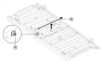
Remove the bolt M and the nut using a 3 mm Allen key and a 7 mm key, to remove the rod M from the bed, and keep all parts available for remounting, when the Soft Tilt is removed again from the bed.
