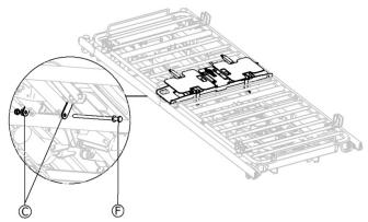
Fix the main module onto the crossbars of the mattress support frame, by placing the carrige-bolt e, trough the designated bracket on the main module e, washer and nut, from underneath on both sides of the bed.
