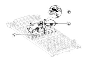
Place the main module © onto the crossbars ®, following the symbol represented in the zoomed image ®. Head facing towards the head end of the bed and feet towards the foot end of the bed.
