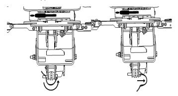
After the pin is removed, the motor will slide out of the support and slowly lower the wing.
